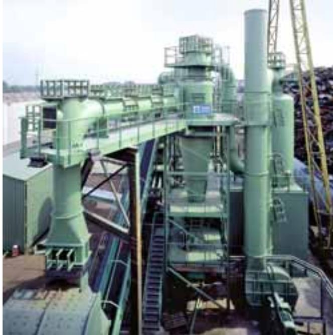
Windsifters, using re-circulated air, are used to clean the mainly ferrous metal scrap for large feed volumes up to 200 t/h. Up to about 90 % of the air is recirculated. The result is a good ferrous scrap quality and low environmental pollution achieved by considerably reducing the volume of air and dust load leaving the equipment.
