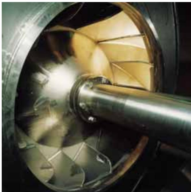
The pressure-shock-resistant fan was specially developed for use in shredder plants. It can withstand pressure shocks up to 3 bar without any great damage to itself thanks to the explosion vents in the fan casing and impeller.
