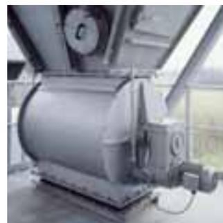
The pressure-shock-resistant and flameproof rotary airlock, developed by Venti Oelde and tested by the Deutsche Montan Technologie GmbH (German Mining Technology Ltd.) in the mining test plant, ensures fire protection isolation, e. g. between filter or separator and the downstream conveying system. The state-of-the-art construction complies with the applicable standards and guidelines.
