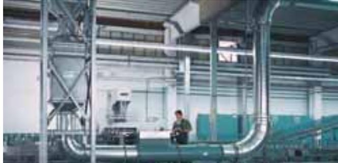
Great emphasis is placed on hygiene in the food-processing industry. For the drinks industry, for example, PET bottles are treated in our suction type PET bottle conveying plant. This makes it impossible for residual liquid or contaminated air to leak from the pneumatic conveyor system.
