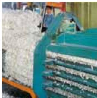
The discharged waste is compressed in bale or container presses. Dust from the filter plants is collected in big bags or compressed to briquettes or pellets.
