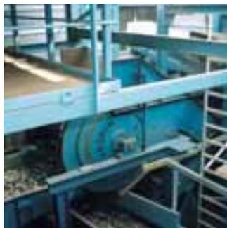
The waste fractions are automatically discharged from the conveyors directly into containers. All conveyor belts for transport of the shredder fluff are covered and can be equipped with additional dust extraction.
