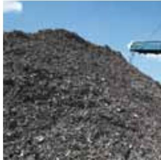
Pivotable discharge belts are used to discharge the ferrous fraction so as to obtain a large stockpile volume.
