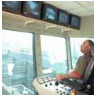
A good example of this is the working method of large shredder plants. Venti Oelde risked a step forward by replacing the control panel by a control cabin in which the shredder operator can sit comfortably and keep an eye on all vital process data and also the shredder infeed area at all times.
